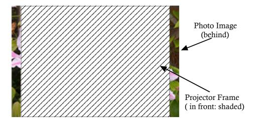
In the figure above the shaded rectangle represents the image frame of the projector, in the proportions 4 wide by 3 high. The image behind represents a normal camera photograph in the proportions 3 wide by 2 high. The two images have been scaled so that they are the same height as the projector frame, so that the full height of the photograph can be displayed. However, the two bits of the photograph visible at either side lie outside the projector's image frame. Hence they are not displayed.
